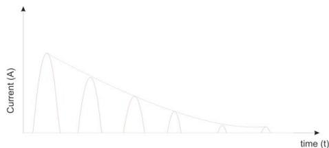
Figure 5: Inrush current transient behaviour
