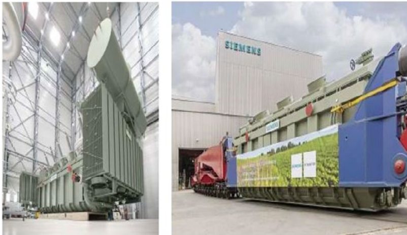
Figure 6. The 300MVA, 420-kV natural ester FR3 filled Power Transformer in the test bay and during delivery.
