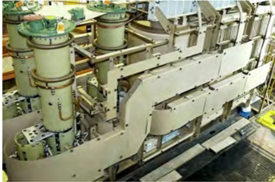
Figure 8: Example of the active part of a large power transformer
