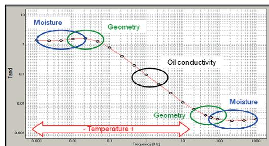
Figure 4. Parameters that effects the dissipation factor at various frequencies
