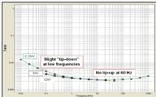
Figure 21. DFR tip-up measurement on bushing #5 (“good”).
