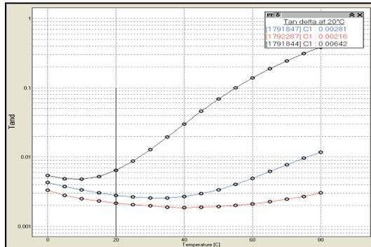
Figure 24. Tan delta temperature dependence, 26 kV GE type T bushings
