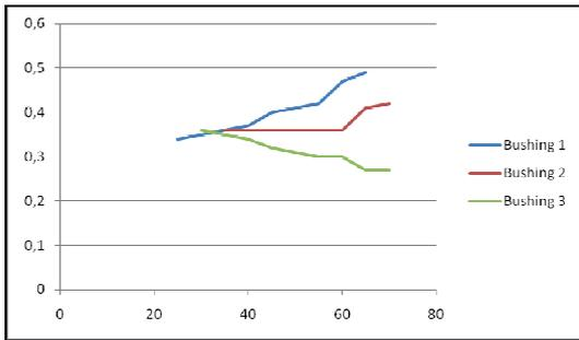
Figure 9. Tan delta values as function of temperature (°C) for three different bushings [10].
