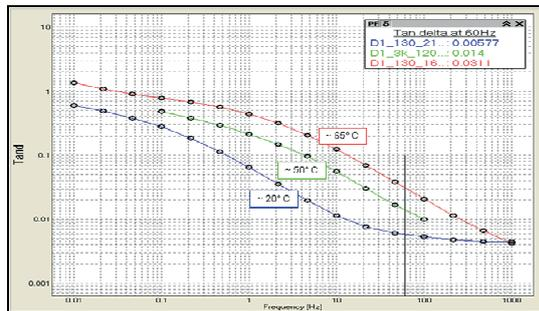
Figure 18. DFR measurement on bushing #1 at different temperatures
