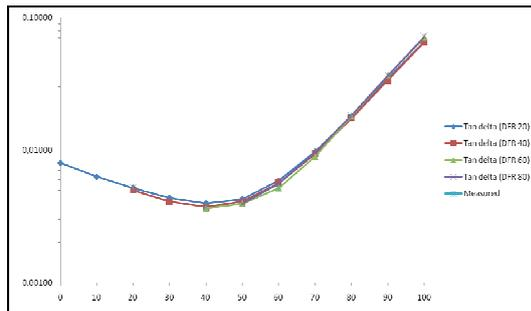
Fig 11. Tan delta at 50Hz for dry Kraft paper as function of temperature
