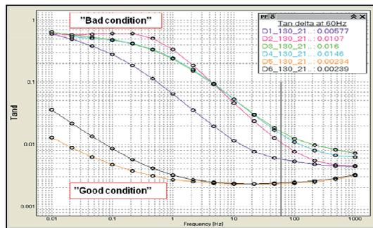
Figure 16. Tan delta vs frequency measured at 0.13 kV and ambient temperature
