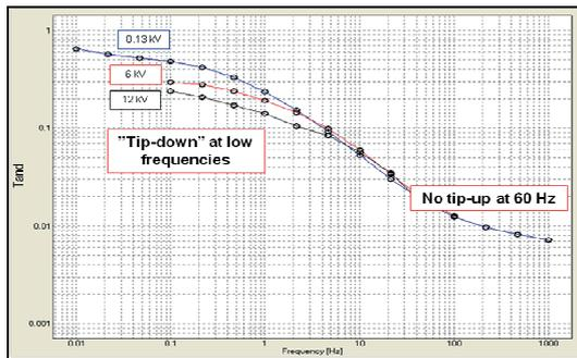
Figure 20. DFR tip-up measurement on bushing #3 (“bad”).
