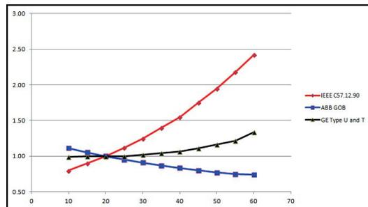
Figure 1. Typical dissipation factor temperature corrections (relative tan delta as function of temperature)
