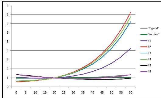
Figure 17. Tan delta temperature dependence (relative tan delta) for the six bushings (temperature on x-axis)
