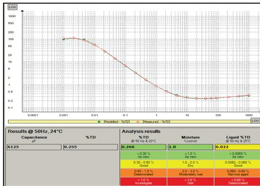
Figure 5. DFR insulation assessment and moisture analysis
