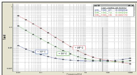
Figure 19. DFR measurement on bushing #5 at different temperatures
