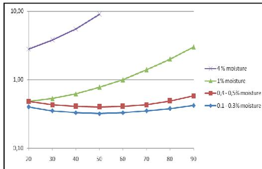
Figure 13. Dissipation factor (%) vs temperature for OIP bushings with various moisture content, [14]
