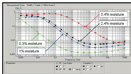
Figure 3. DFR measurements on four different transformers at different temperatures with moisture content ranging from 0.3 to 3.4%
