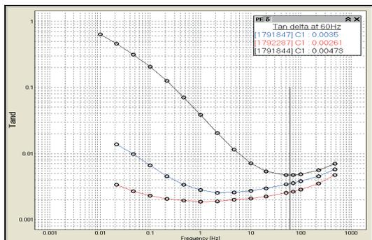
Figure 23. C1 DFR measurement on 26 kV GE type T bushings
