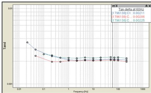
Figure 22. C1 DFR measurement on 220 kV GE type U bushings
