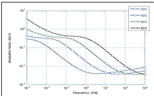
Fig 10. Dissipation factor as function of frequency for dry Kraft paper.
