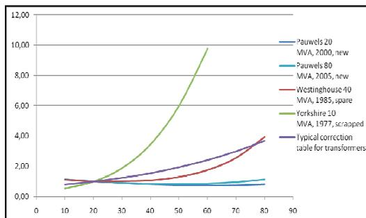
Fig 12. Temperature correction for transformers in various conditions
