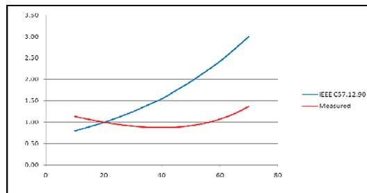
Figure 22. Individual tan delta temperature correction (ITC) compared to IEEE C57.12.90 temperature correction table (TCF)
