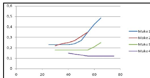
Figure 8. Tan delta values as function of temperature (°C) for four different transformers [11].
