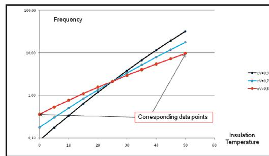
Figure 7. Relationship between power factor values at different frequencies taken at different temperatures.
