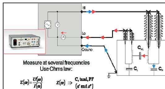
Figure 2. DFR/FDS test setup
