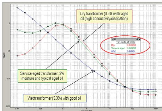
Figure 6. DFR analysis for three transformers with different oil quality and moisture content
