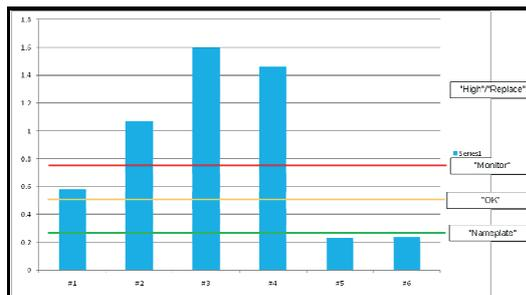
Figure 14. Dissipation factor (%) for the six GE Type U bushings at 20°C
