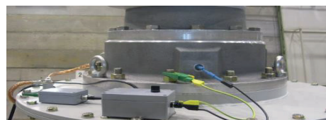
Fig. 7: Quadrupole and preamplifier fitted to the tap
