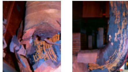
Figure 7: Connection of LV winding to LV bushing at a 181 MVA generator step-up transformer with obvious signs of pyrolysis
