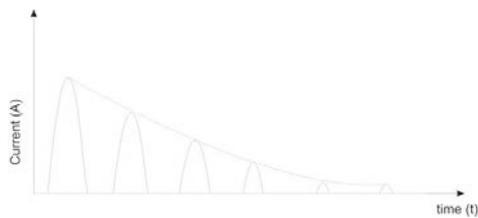
Figure 5: Inrush current transient behaviour
