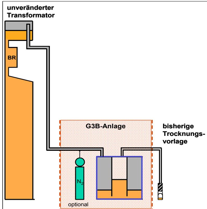
Figure 5: Principal scheme of the breather buffer box
