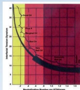
A precise classification of transformer insulation oils involves the unique relationship between interfacial tension (IFT) and neutralization number (NN). Several IFT studies show that an increase in NN should normally be followed by a typical drop in IFT. If the values of IFT versus NN for a given oil sample do not fall within a reasonable range on either side of the median line, further investigation is in order.
