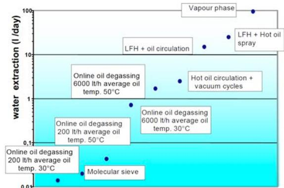
Figure 14. Drying velocity from 3% down to 1,5 % average humidity
