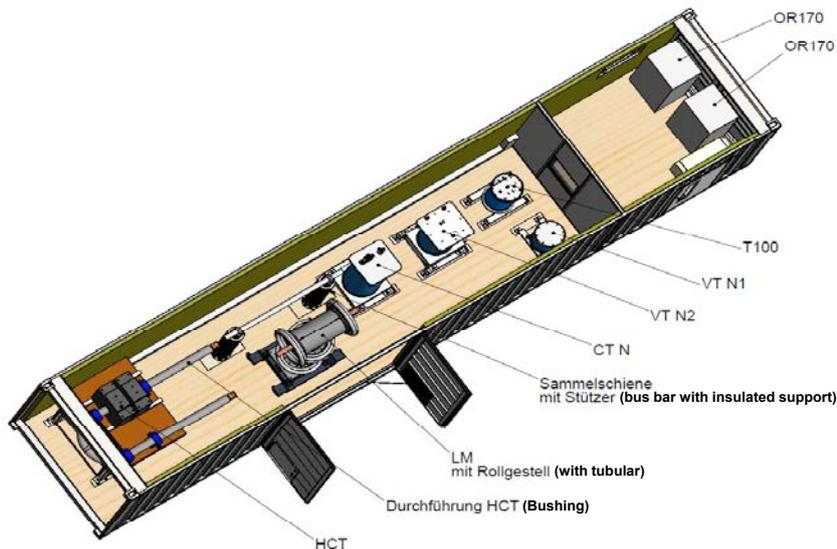
24.07.2013 A New Generation of a Loss Measuring System for Power Transformers
