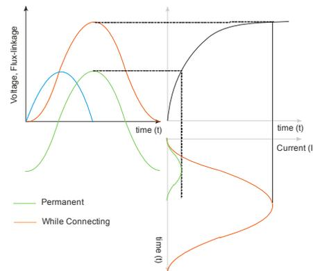
Figure 3: Voltage-currents while connecting and in permanent cycle
