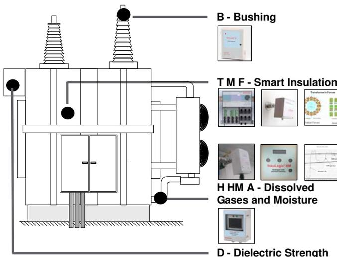
Monitors & Software to optimize transformer operation
