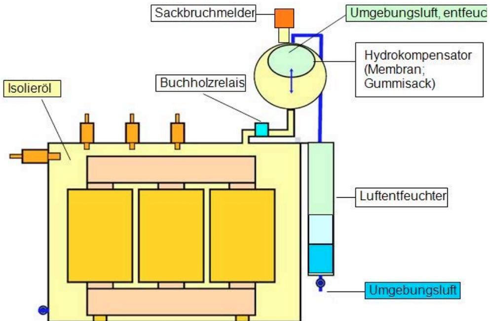
Figure 3: Transformer with hydro-type compensator
