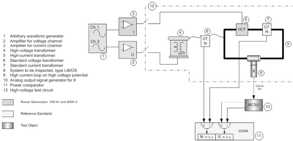
24.07.2013 A New Generation of a Loss Measuring System for Power Transformers
