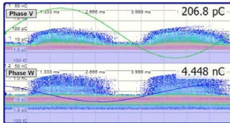
**Figure 8:** Electrical PD pattern recorded at the bushing taps of phases V and W
