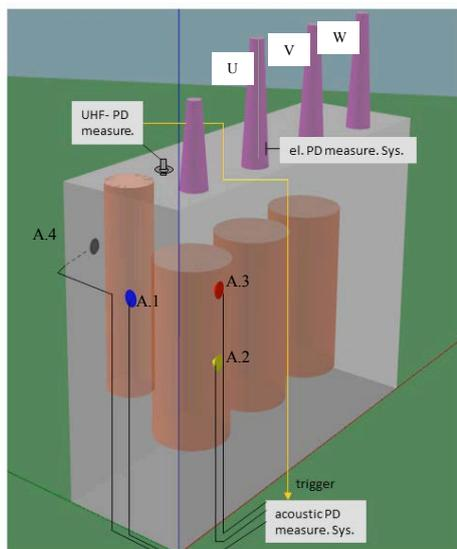
**Figure 14:** Test setup (UHF, el. and acoustic PD)
