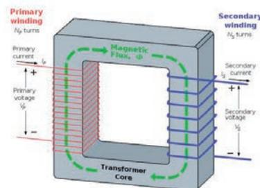
Fig 1. Transformer function sketch
