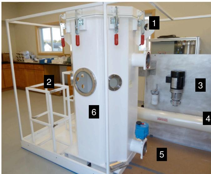
1. Transformer simulation tank with removable cover, surrounded by safety frame
