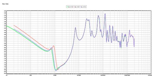
As expected FRA trace moves left, back to the original status after application of the demagnetization algorithm.
