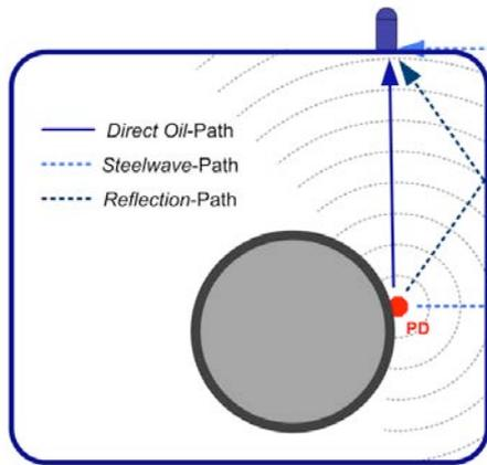
**Figure 1:** Possible propagation paths in the test object [5]
