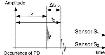
**Figure 3:** Absolute and relative times in a two-sensor-setup
