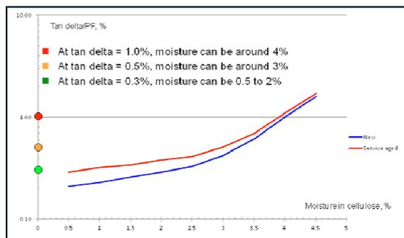
Figure 9. Tan delta (% @ 20C) vs moisture (%) for a new and service-aged typical core-form transformer
