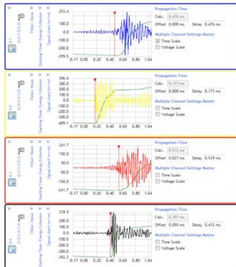
**Figure 9:** Acoustical PD signals detected during the location procedure
