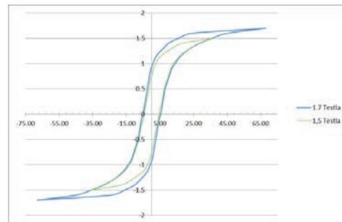
Figure 2: Hysteresis loop of grain oriented magnetic steel
