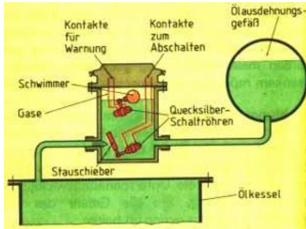
Figure 11: Principal construction of the Buchholz relay
