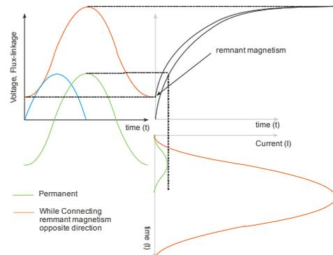
Figure 4: Voltage-currents while connecting and in permanent cycle, remnant magnetism opposite direction
