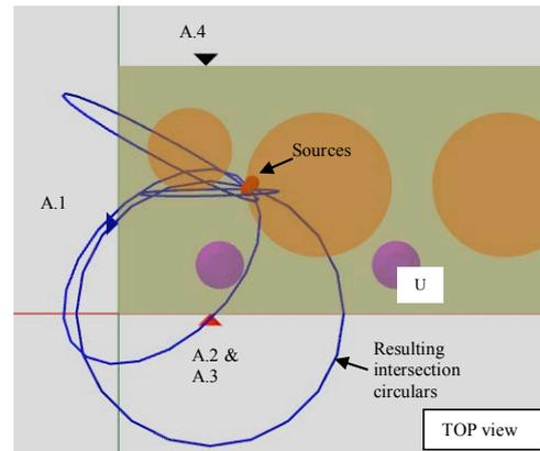
**Figure 15:** Estimated PD source location and some intersection circulars
