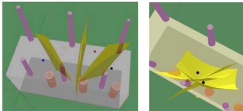
**Figure 17:** Results with initial sensor placement (left) and after sensor-repositioning (right). PD source indicated to be close to the tap changer or MV bushing of the middle phase.
