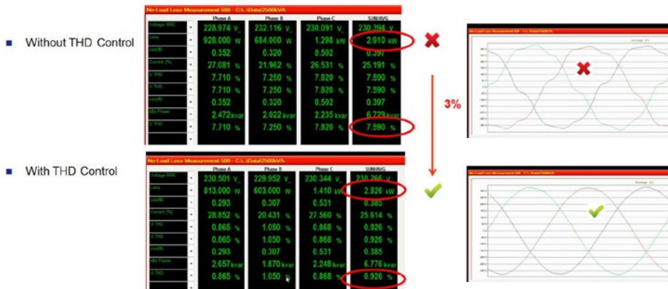
Fig. 1. (a) THD impact on no load loss on a 2.5 MVA transformer
