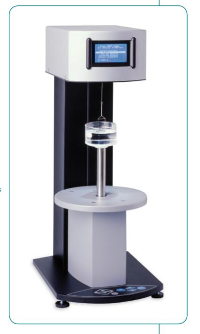
The SIGMA 2000 interfacial tensiometer is a fully automatic device for the measurement of interfacial tension in transformer oil accord. to ASTM-D971 and IEC60422. No previous knowledge of IFT measurement is required, the step-by-step instruction on the large LCD display guides you through the measurement process and ensures fail-safe measurement every time.
